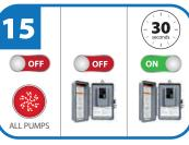
Turn off all pumps. Then turn main power off to the spa for 30 seconds. Then turn power back on.
