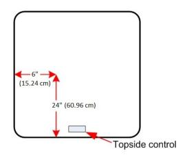
FIGURE 1: ELECTRICAL CONDUIT LOCATION
