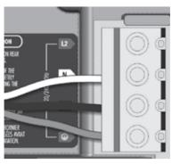
Connections for 120 V heaters (1 kW)
