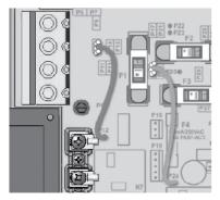
Note: To convert model to a 120 V system, the white (common) accessory wire must be moved. See wiring diagram for details.
